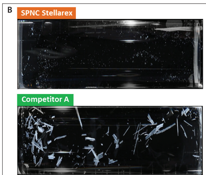
Figure 1. Total particulate loss after balloon inflation in a vessel of room temperature water (A). Photo display of the particulate generated after a balloon is submerged in a vessel of room temperature water, inflated to nominal pressure, and removed from the vessel (B).
